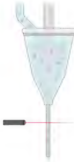
Figure 29. Schematic illustration of Flow Cytometry. A laser beam going through the pipe containing the sample with vesicles. The vesicles pass the light one by one. The scattered light can be detected and analyzed.
